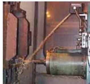
Inadequate coolant delivery
